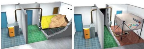
TRANSFERT PAR ASPIRATION AVEC SILO MAÇONNÉ OU SILO EN TOILE © ÖKOFEN
