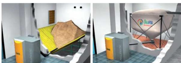
TRANSFERT PAR VIS AVEC SILO MAÇONNÉ OU SILO EN TOILE © ÖKOFEN
